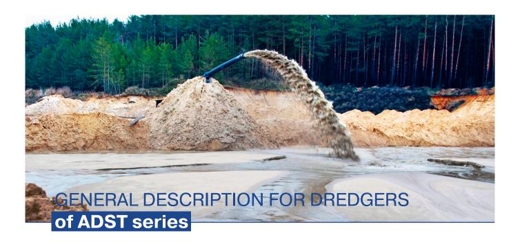
The dredgers of the **ADST** series are based on the concept of dredging with a submersible pump that is specifically designed for high viscosity mixtures and high solids content mixtures. There is no need to equip the dredger of the **ADST** series with a ladder carrying the dredging system (i.e., suction pipeline and ripper).
