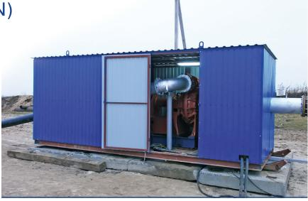
The complex, controlled by one workplace, fully automatically operates with the ability to pumping sand-gravel slurry up to one kilometer without breaking a jet. The hydraulic and mechanical complex includes booster pumps for hydraulic ripping in the soil intake area for dredge operation.
